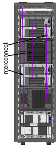
Figure 23 Chassis to Chassis within the Same Rack Interconnect Application Space
